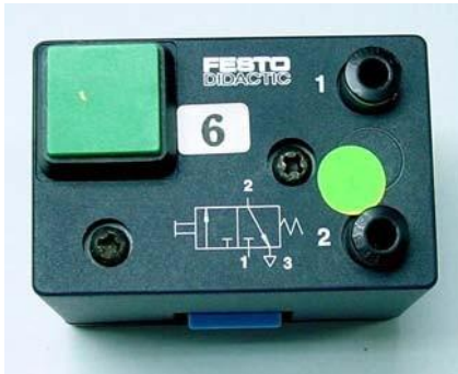
Fig. 40 (a) 3/2 Directional control valve
