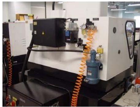
(b) Pneumatic system of an automatic machine
