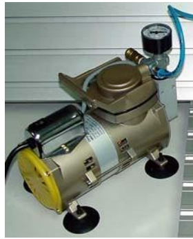
(a) Compressor used in schools (b) Compressor used in laboratories (c) Pneumatic symbol of a compressor
